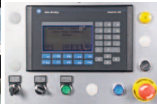
Control panel SBV 1200.
