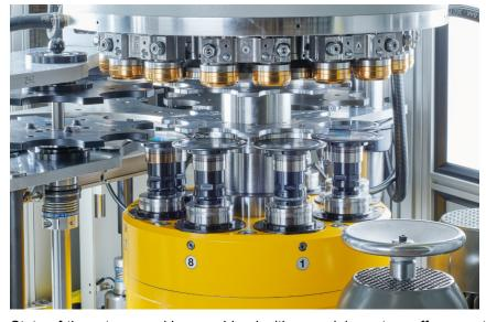
High-end design with a completely enclosed lubrication circulation and the well known proven technical reliability **GERMANN FREI** machines, make the seamer low maintenance. CSM 800 equipped synchronized can stop turret. The flexible synthetic material and scratch avoiding hard-chromed guiding parts enable a gentle can handling. The discharge is set at 180° to inlet and offers the full flexibility for further transportation direction.
