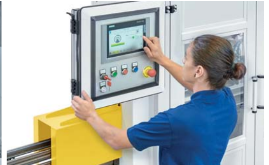
Simple operation of the PLC via an HMI touch panel
